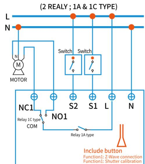
Example 2, connecting a DC Track curtain motor.
