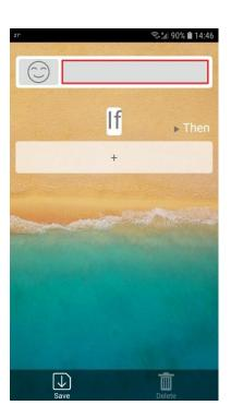
Enter your desired name for your Marco in the Top bar (in this example Smart Button) and press "OK". Now add the "IF" device to the Macro, Press the "+" symbol and a list of devices will appear now select your "Smart Button" from the list. After the Smart Button has been added click on ">0" behind the Smart Button.
