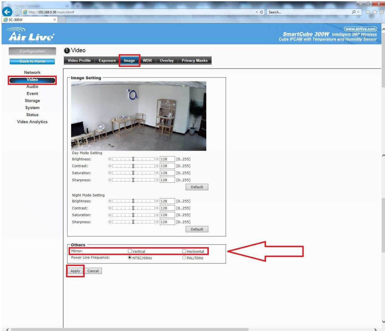
After the settings have been adjusted you need to press “ Apply “ to save the settings.
