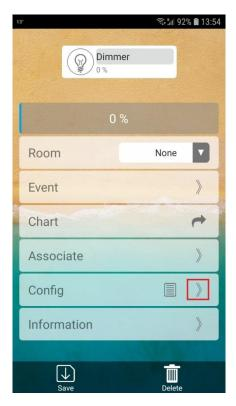
The default function of both S1 and S2 is "One Switch mode". In the "Config" menu of the SD-101 this can be changed to either "Two Switch mode or UP/Down Switch mode. The Parameter to change S1 and S2 is Parameter 3. The Value is default 1 (One switch mode). Please see the table and description below.
