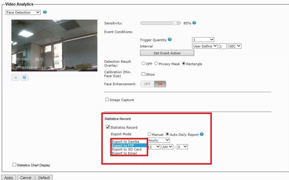
5. Enter your FTP information and select the time for the report to be send. Press “ Test FTP” to test your FTP connection. After this was successful press “ Apply” to save your settings.
