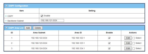
You can enable the OSPF routing function by click on the "Enable" button for OSPF item. There are 8 area subnets can be defined in the OSPF network and enable them individually. When you finished setting, click on "Save" to store your settings. Above settings are just for examples.
