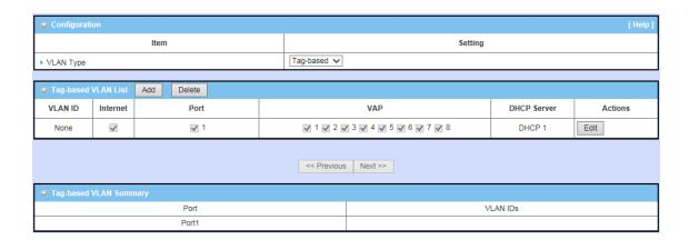
By default, all the LAN ports and virtual Aps belong to one VLAN group, and this VLAN ID is forced to "1" but noted as "None" for avoiding misunderstanding. It is a special Tag-based VLAN group for the Intranet of device to operated, there is not a required in Intranet packets for this default VLAN group with that ID. Also be noted, there is only one Ethernet LAN port in the device.
