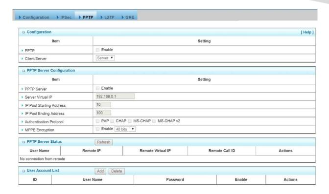
PPTP: Check the "Enable" box to activate PPTP client and server functions.
