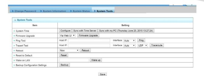
1. System Time: There are three approaches to setup the system time. Before the process, some basic information must be filled by clicking on the "Configure" command button. Basic information includes following items:
