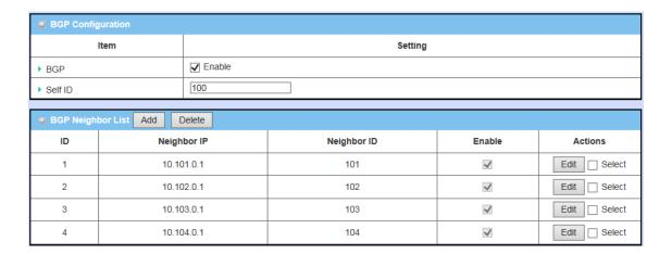
You can enable the BGP routing function by click on the "Setting" button and fill in the corresponding setting you're your BGP routing configuration. When you finished setting, click on "Save" to store your settings or click "Undo" to give up the changes. Above settings are just for examples.
