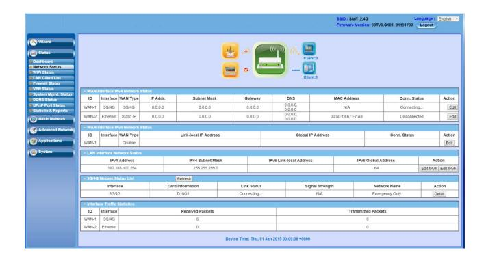
**Note:** You can see the first screen is located at **[Status] - [Network Status]** after you logged in and the screen shows the Network Connection Status below.
