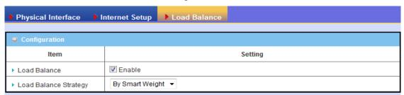
Load Balance: Enable or disable the load balance function.
