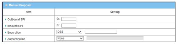
When "Manually" key management is used, there are 4 further parameters need to be specified by you and used in IPSec tunnel establishing.
