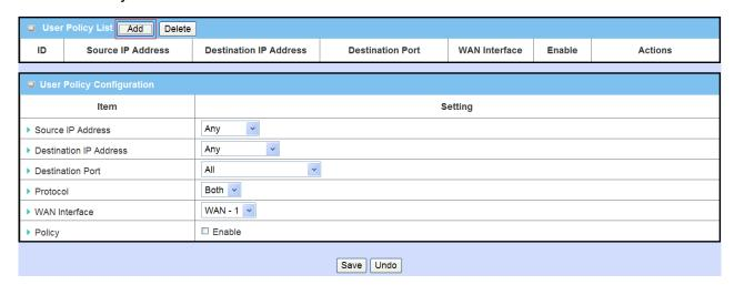
**Source IP Address**: Enter the expected Source IP Address for the load balance policy. It can be "Any", "Subnet", "IP Range", or "Single IP". Just choose one type of the source IP address, and specify its value as well. If you don't want to specify a certain source IP address for this policy, just leave it as "Any".
