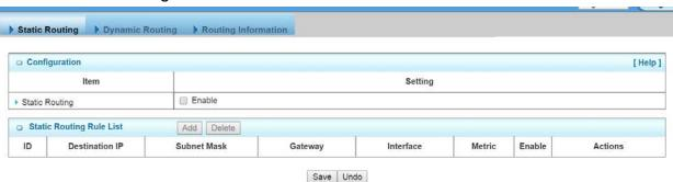
For static routing, you can specify up to 32 routing rules. The routing rules allow you to determine which physical interface addresses are utilized for outgoing IP datagrams. You can enter the **destination IP address**, **Subnet Mask**, **Gateway**, and **Metric** for each routing rule, and then enable or disable the rule by checking or un-checking the Enable checkbox.
