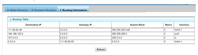
A routing table, or routing information base(RIB), is a data table stored in a router or a networked computer that lists the routes to particular network destinations, and in some cases, metrics(distances) associated with those routes. The routing table contains information about the topology of the network immediately around it.
