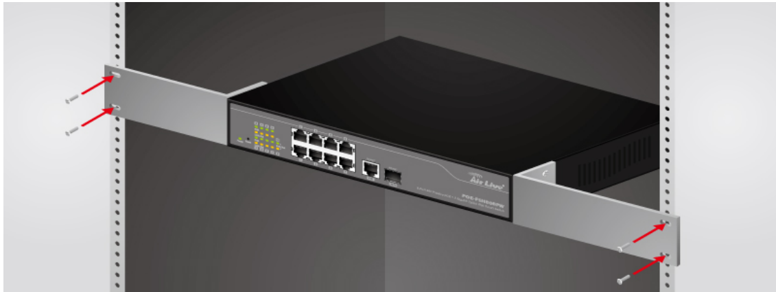
Attaching the Switch to a 19-inch rack
