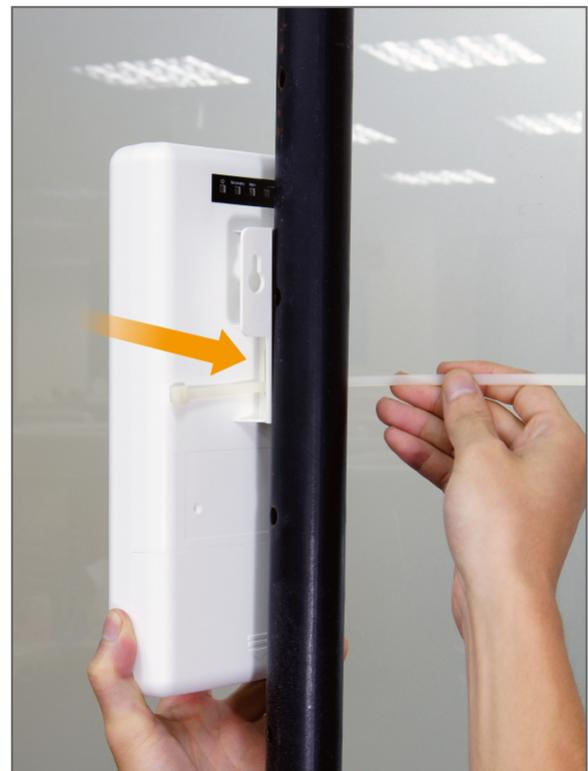
2. Thread the thinner end of the strap into the opening on the other end. Then tighten the strap around the pole as tightly as possible.
