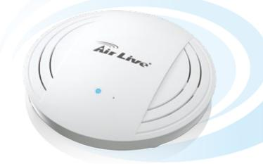
A irLive AC.TOP is MIMO 802.11 a/b/g/n/ac Ceiling AP with data rate up to 1200Mbps which is ideal for wireless video streaming or video gaming. Ceiling mount type AC.TOP with high power also provides wide coverage. It built-in IEEE 802.3af PoE to deploy the PoE network environment that reduces the complexity wiring and easy- to-install into the existing network environment. With different wireless modes, AC.TOP not only fully fulfills to different application but also expand wireless coverage.
