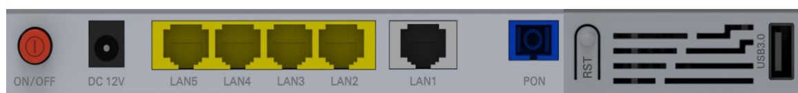
Figure 4. Interface/button Panel, RST and USB on the side of the device.
