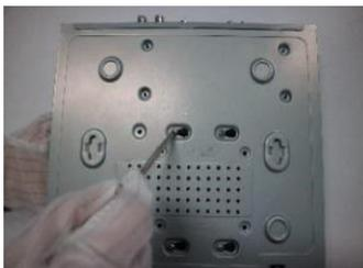
3. Slide the hard drive into the screw slots. Tighten all screws.
