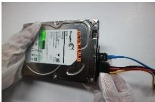
2. Tighten the 4 screws through hard drive screws holes, connect the data and power cables
