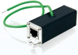
POE Surge Protectors such as AirLive SP-100E can protect your IPCAM from power surge and ESD from lightning. The SP-100E is highly recommended for outdoor camera installations. Please make sure the SP-100E's green cable is properly grounded
