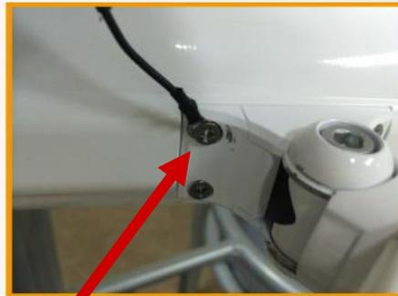
**Secure one end of ground cable to the screw on the mounting.**
