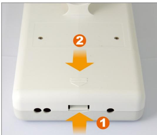
2. Pass through Ethernet cable from the hole; insert the cable to Secondary port.
