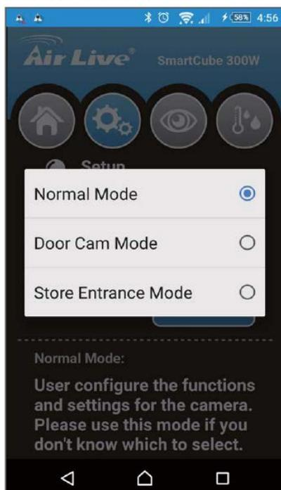
8. You can adjust resolution, frame rate and PIR motion detection in normal mode.
