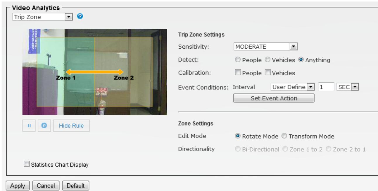
1. Select **Sensitivity** to set the detection sensitivity level. Higher sensitivity will make it easier to detect and less objects missing, but more misjudgments.
