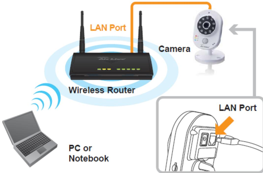
**Note:** If you want to connect your PC directly to the camera by Ethernet cable, the IP camera's default LAN port IP address is 192.168.1.100.
