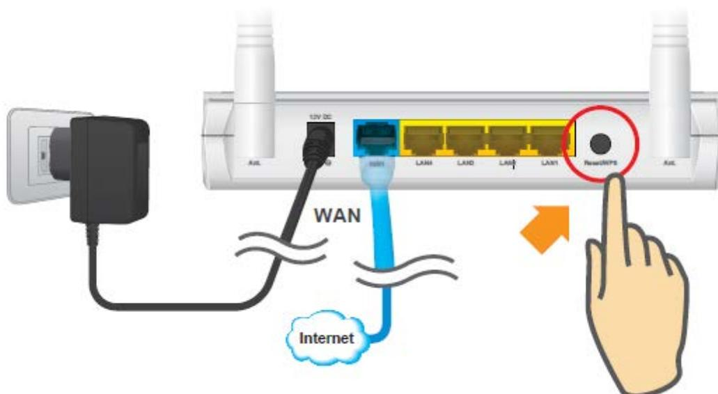
2. Click Reset/WPS button on SmartCube 300W then the green led will be on for 2 minutes. When SmartCube 300W connects to the router successfully, the green led will be flashing.
