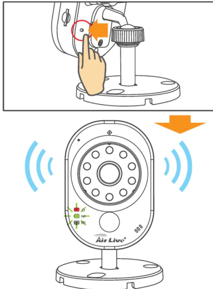
**Note:** The WPS function only works when the router is in WPA2 AES security protocols or has no protected password.
