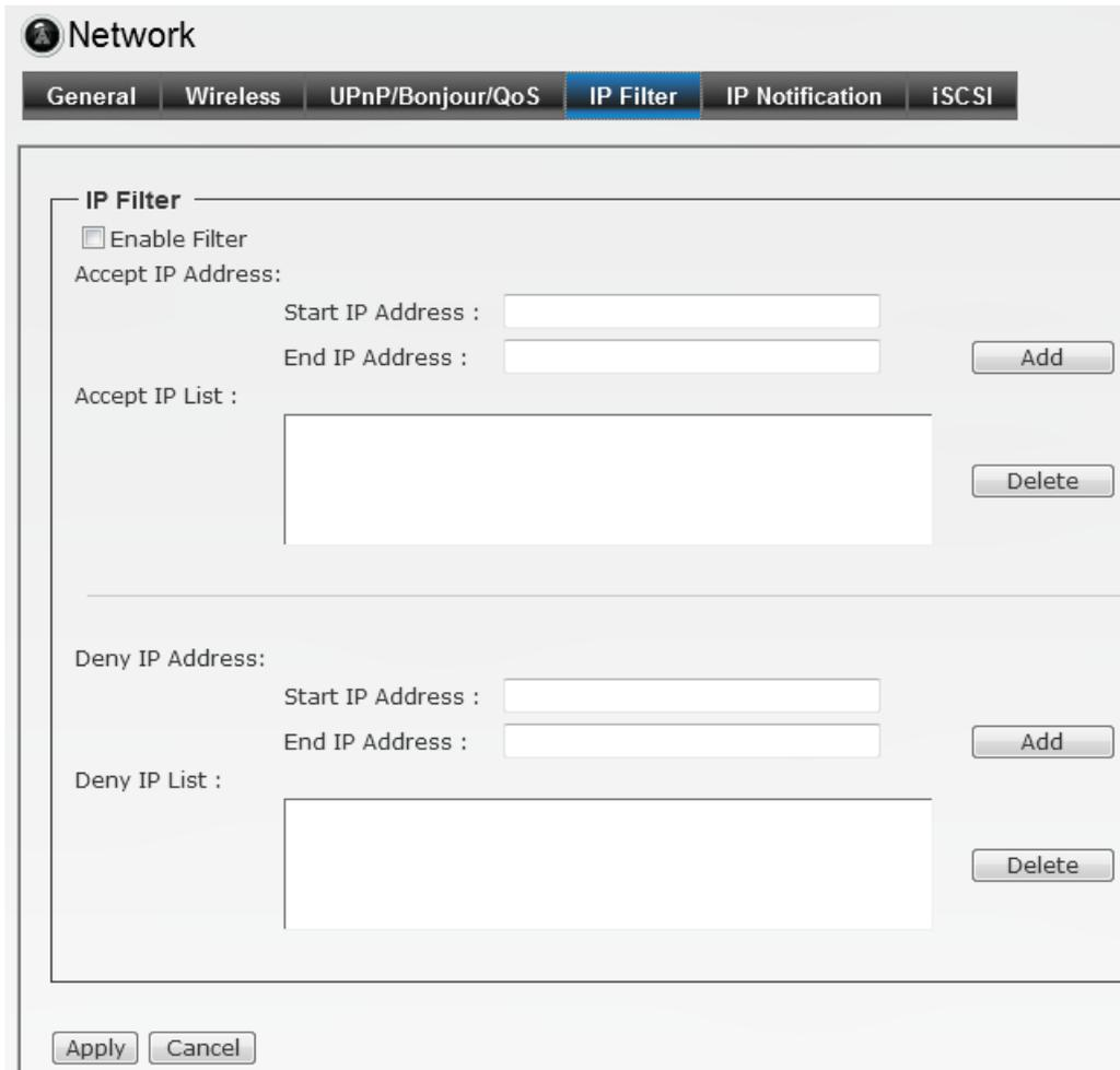
The screenshot shows the 'Network' configuration page with the 'IP Filter' tab selected. The 'IP Filter' section includes an 'Enable Filter' checkbox. Below it are two main sections: 'Accept IP Address' and 'Deny IP Address'. Each section has 'Start IP Address' and 'End IP Address' input fields, an 'Add' button, and an 'Accept IP List' or 'Deny IP List' text area with a 'Delete' button. At the bottom of the page are 'Apply' and 'Cancel' buttons.
