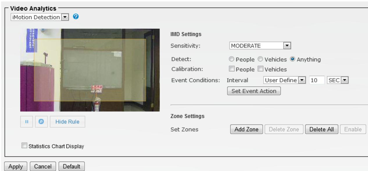
1. Select **Sensitivity** to set the detection sensitivity level. Higher sensitivity will make it easier to detect and less objects missing, but more misjudgments.
