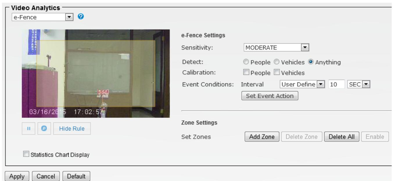
1. Select **Sensitivity** to set the detection sensitivity level. Higher sensitivity will make it easier to detect and less objects missing, but more misjudgments.
