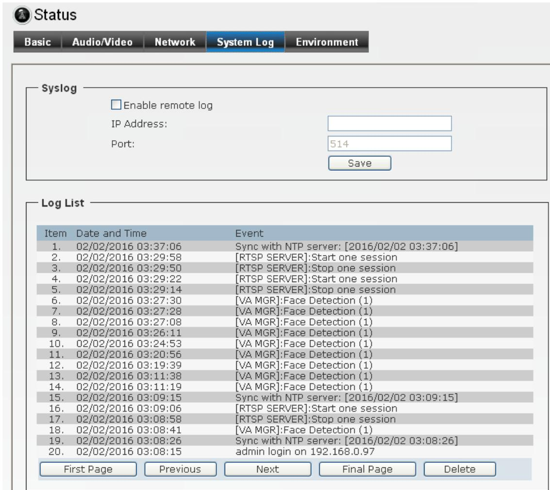
The screenshot shows the 'Status' page with the 'System Log' tab selected. It includes a 'Syslog' section with an 'Enable remote log' checkbox, an 'IP Address' input field, a 'Port' input field (set to 514), and a 'Save' button. Below is a 'Log List' table with 20 entries.
